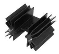
Smart Heatsinks, Inc. introduces the low cost, vertical mount, F - series, standard heat sinks for single and dual TO-247, TO-220 and TO-218, devices. This simple heat sink can hold one TO device with adjustable height, and can be mounted simply by soldering onto PCB. The heat sink has two types of surface finishes, and can be used in either natural (free) or forced convection cooling applications. Cross reference to AAVID P/N: 529701B02100G Series
